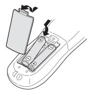
The batteries will last about six months with normal use. If the functions of the remote control unit become erratic, replace the batteries.
